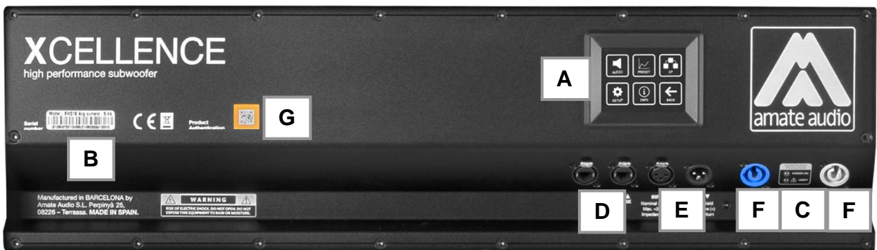
Fig. 10. XW218 control and connection panel
